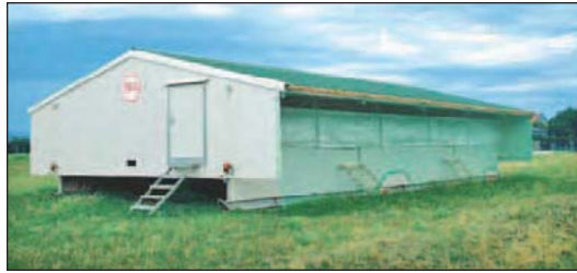
This mobile house has a roofed veranda with curtains that can be lowered in cool weather. Photo by SKA
